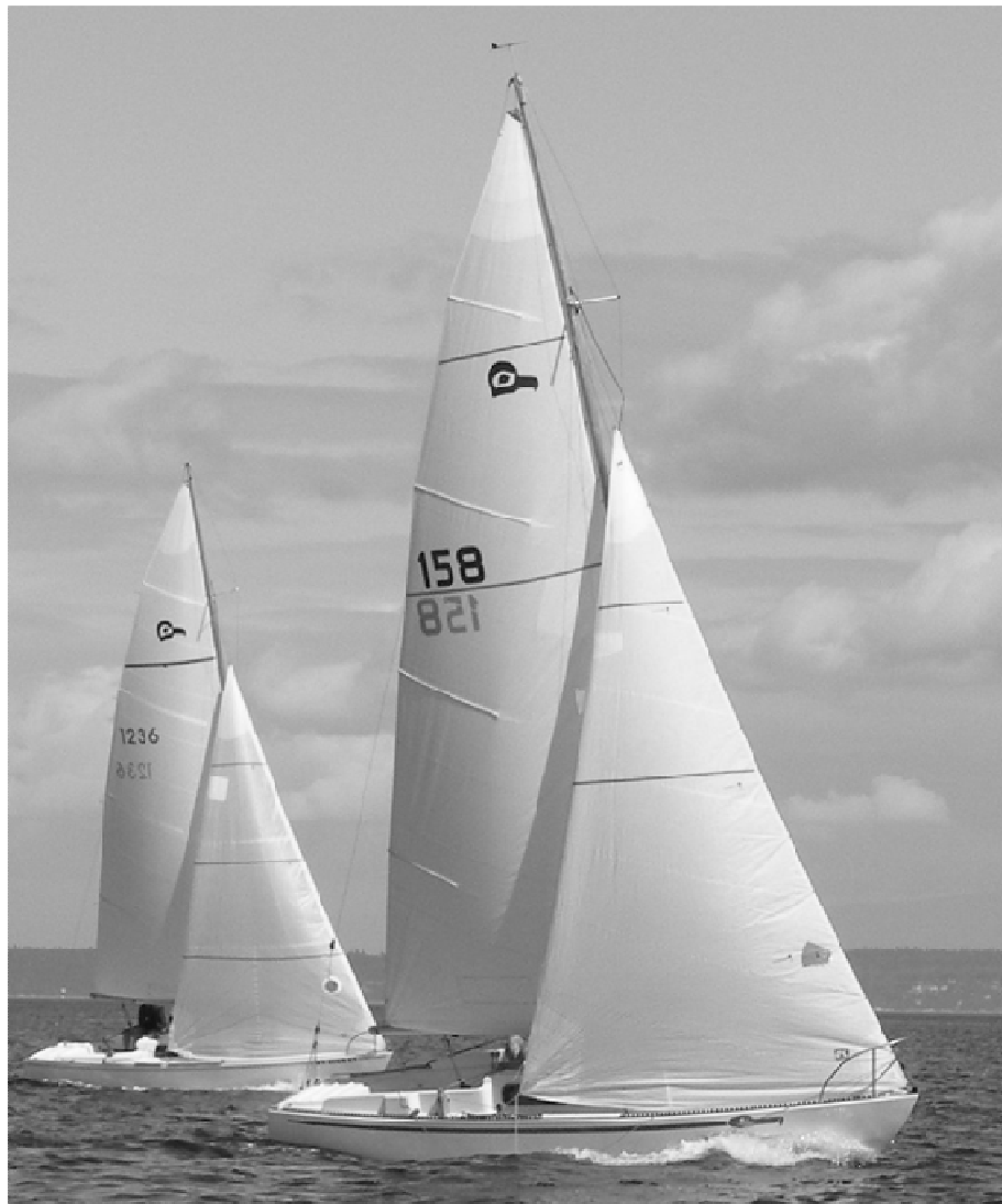
Scooter and Raptor during the Pacific Northwest Regional Championships— Note Scooter's (158) sharp Genoa leading edge for pointing and slacked main outhaul that produces a powerful slot between Genoa and main sails.
